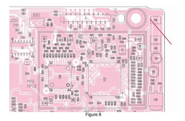
To power the buffer/amplifier, I found a 12 volts power connection from a PCB pad on the PLL PCB (Fig. 8).
